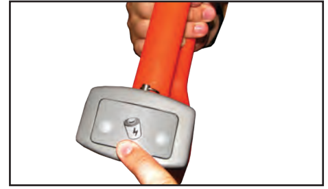
Install four new elements into the battery compartment of the device, minding polarity. Install the battery compartment into the body until it snaps.
