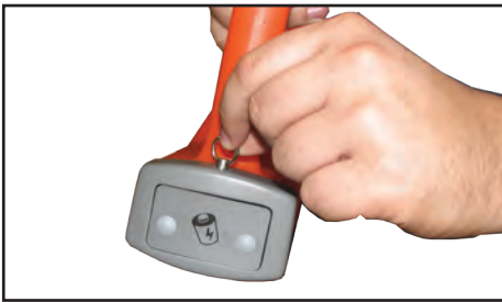
Unsnap Battery compartment. Pull out the ring on the receiver handle.
